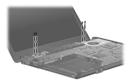
Where used: 4 screws that secure the display assembly hinges to the computer
